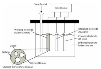
Figure 1. Schematic diagram of the biosensor.
