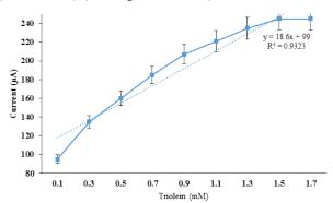
Figure 5. Calibration curve for the developed biosensor.
