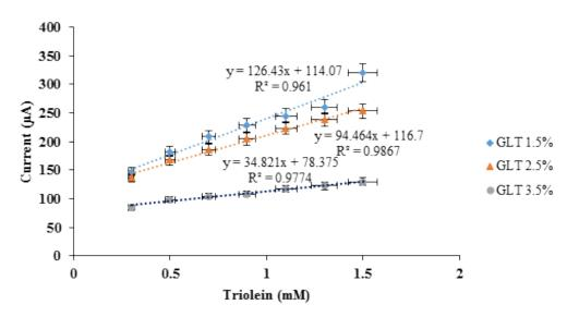
Figure 3. The effect of glutaraldehyde content on biosensor response.
