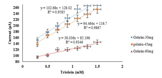
Figure 2. The effect of gelatine content on biosensor response.
